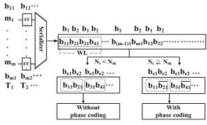
Fig.3: ETI coding scheme for one serial link
