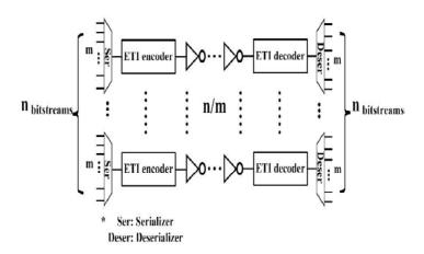
Fig.2: n/m ETI serial link with n input bit streams under degree of multiplexing m.
